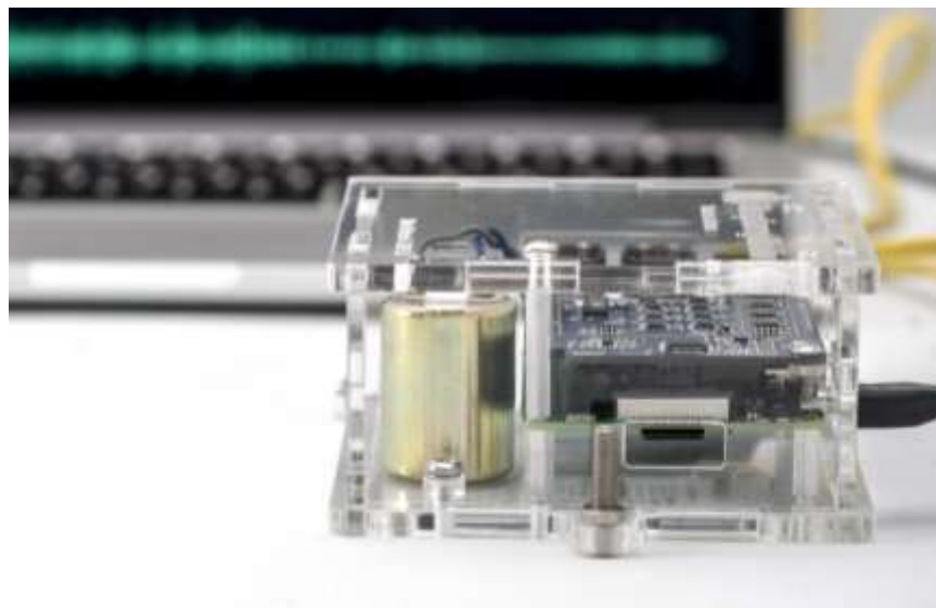
Figure 1. A Raspberry Shake seismograph in a standard clear acrylic case. The brass cylinder frame on the left side of the case contains the geophone. The green board in the case is the Raspberry Pi computer, and the Raspberry Shake header board sits atop it. If the device contains accelerometers, they are contained in chips that are mounted atop the header board. Leveling feet
